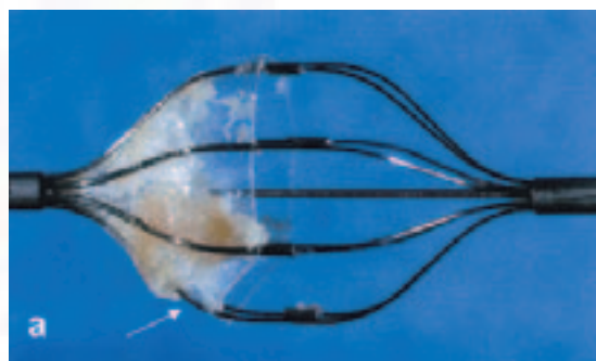
Figure 1. Thrombotic material captured by a Cordis Angioguard™ device. Arrow points to a fold in the plastic membrane which occurred during the retrieval of the protection system.
