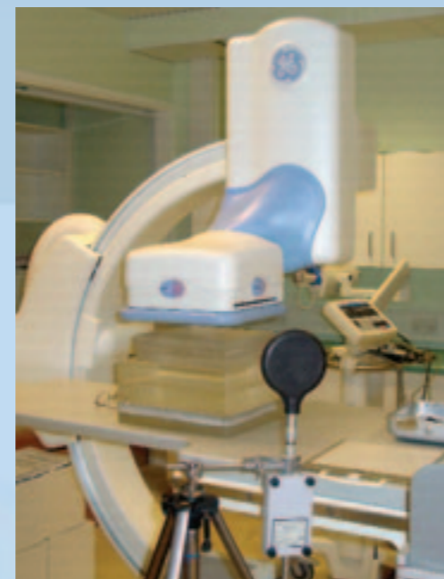
Figure 1. Scatter simulation in a cardiology laboratory. A stack of polymethyl methacrylate (similar in atomic number and density to tissue) is used to simulate the patient and radiation measurement is made with a large volume ionisation chamber.
